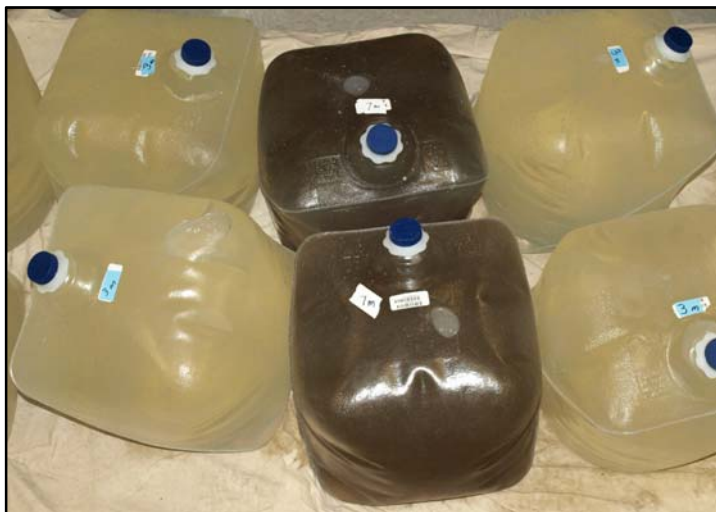
Fig. 23. 10-L containers of water collected from the mixed layer (3 m) and the deep brine layer (7 m) of Gilbert Bay on October 16, 2009. The deep brine layer water contains high concentrations of dissolved organic material, suspended detritus, and toxic hydrogen sulfide and methyl mercury.
