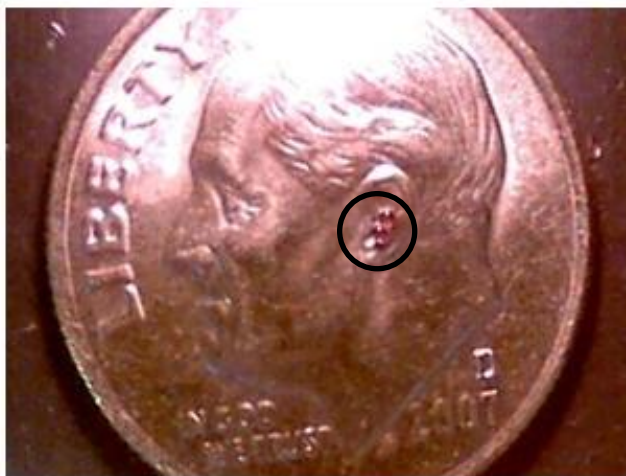
FIG. 2.17. Isolating sapphire spheres (0.5mm diameter). Sapphire sphere shown in Roosevelt's ear for scale.
