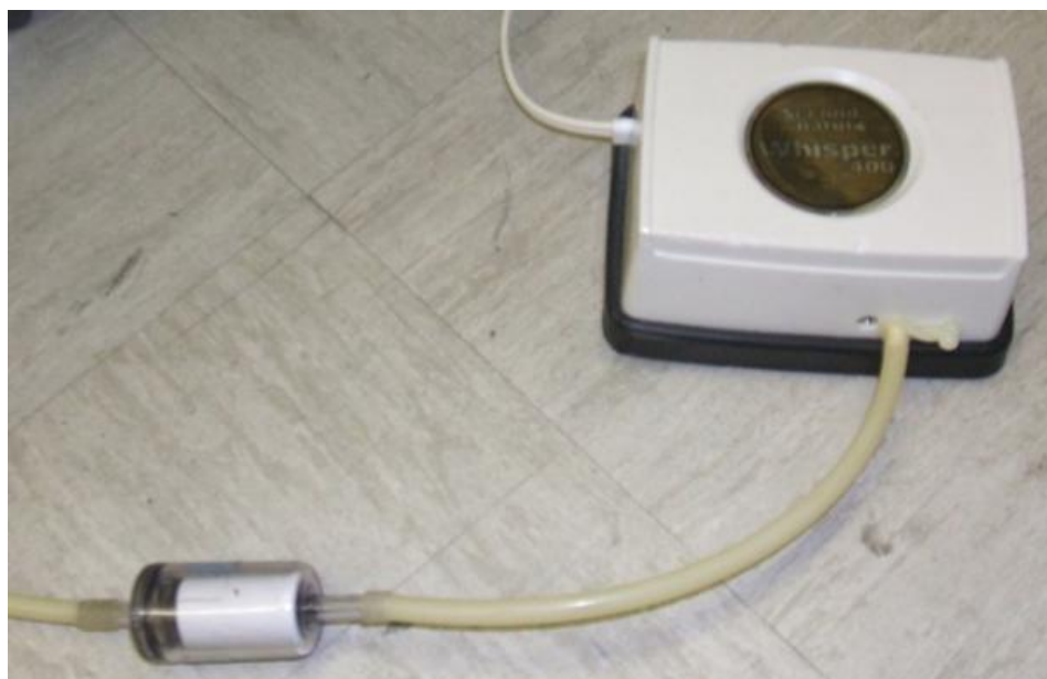
FIG. 2.9. Dry air purge pump and desiccant filter.
