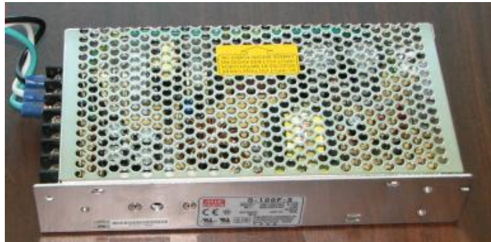
Fig. 14 Mean Well 5V 20-amp voltage regulated power supply.
