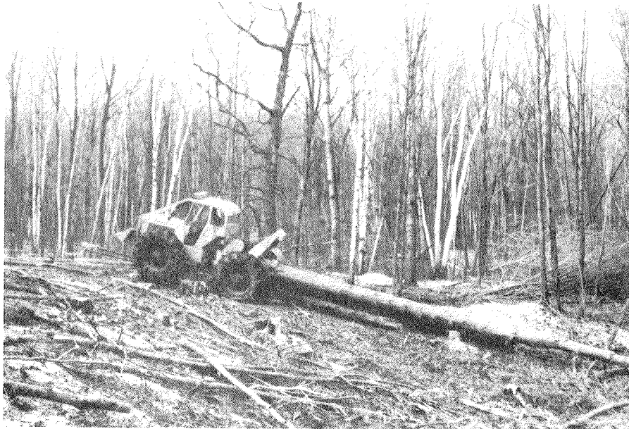
Figure 5. A rubber-tired skidder dragged the tree-length logs to the landing.
