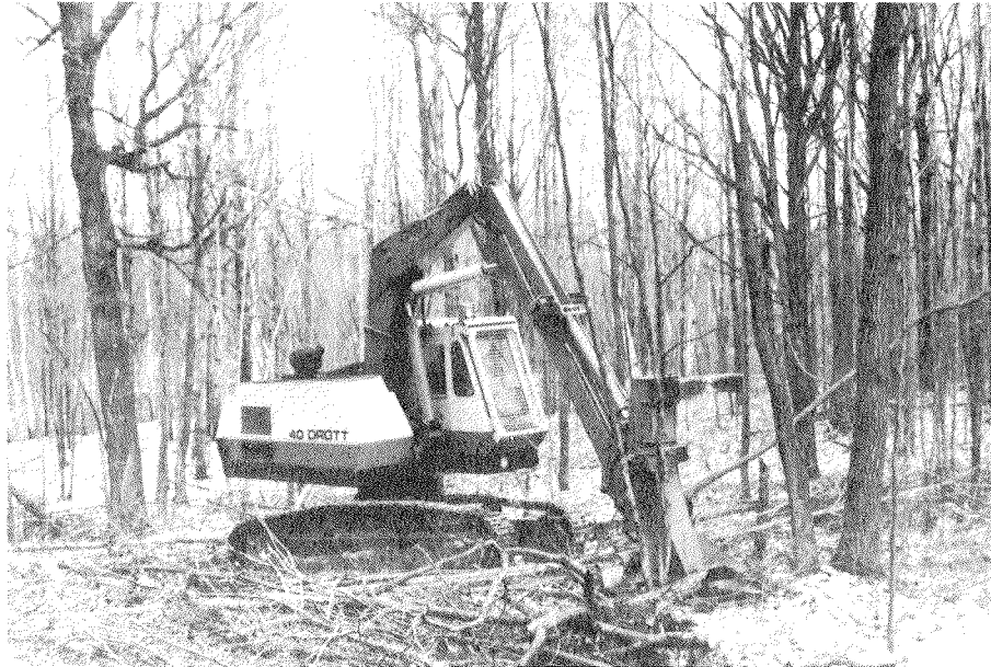
Figure 3. This felling and bunching machine was used in the harvesting operation.
