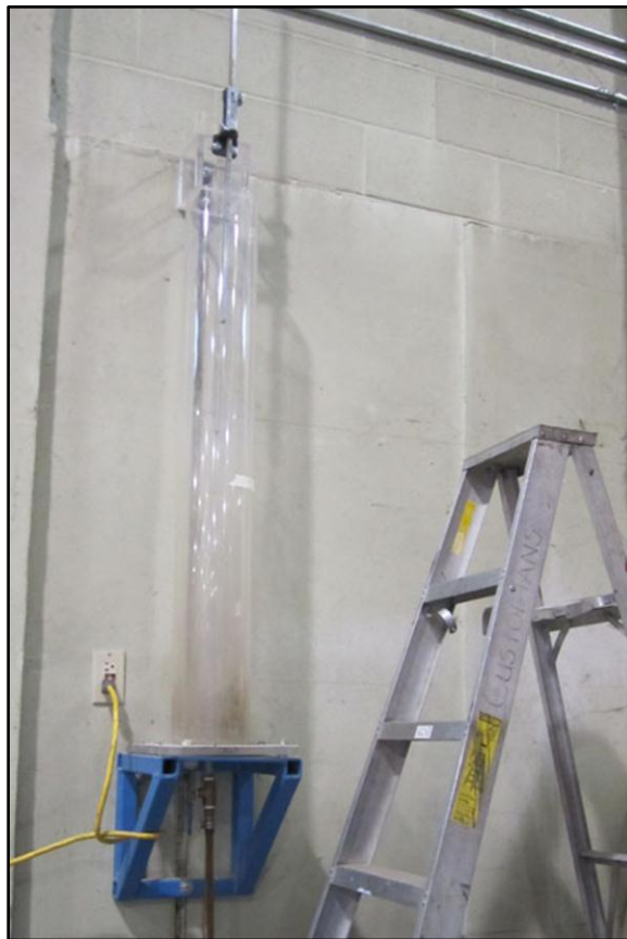
Fig. 14. Stilling basin & point gauge.
