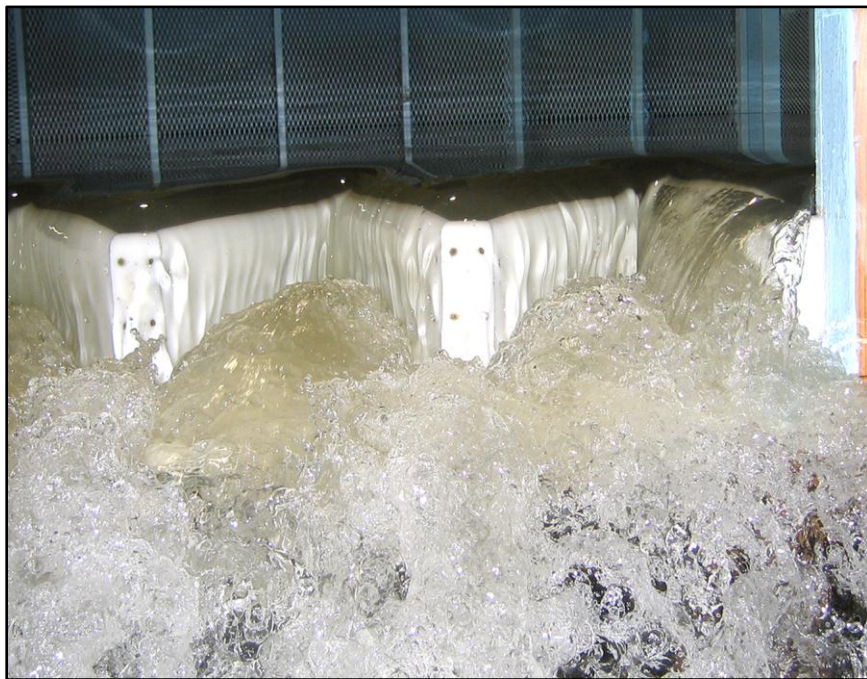
Fig. 24. Natural aeration of 0.5 cycles on \alpha = 20^\circ sidewalls ( H_T/P = 0.2 ).
