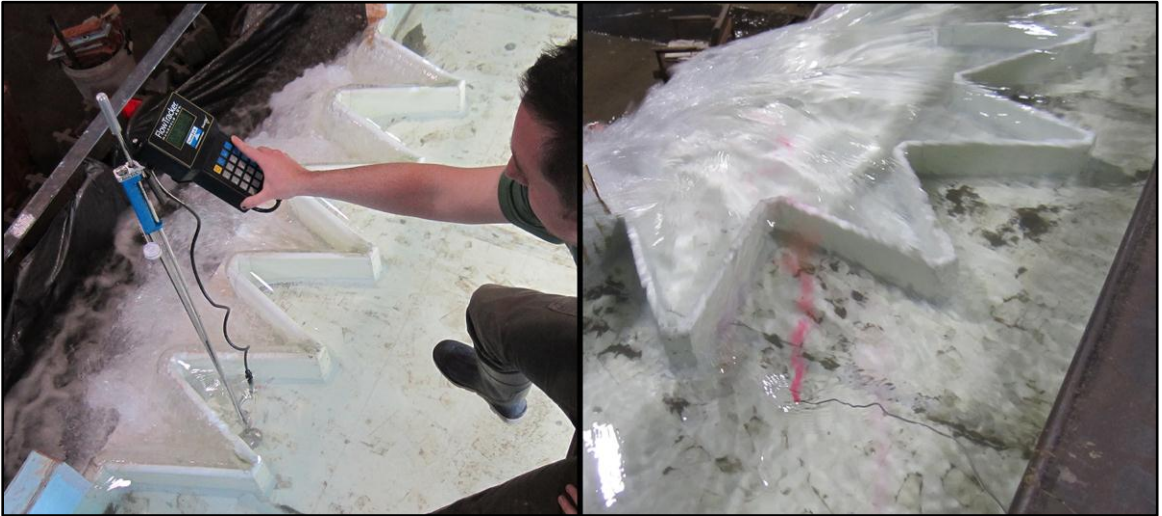
Fig. 15. Velocity probe & dye wand injection.
