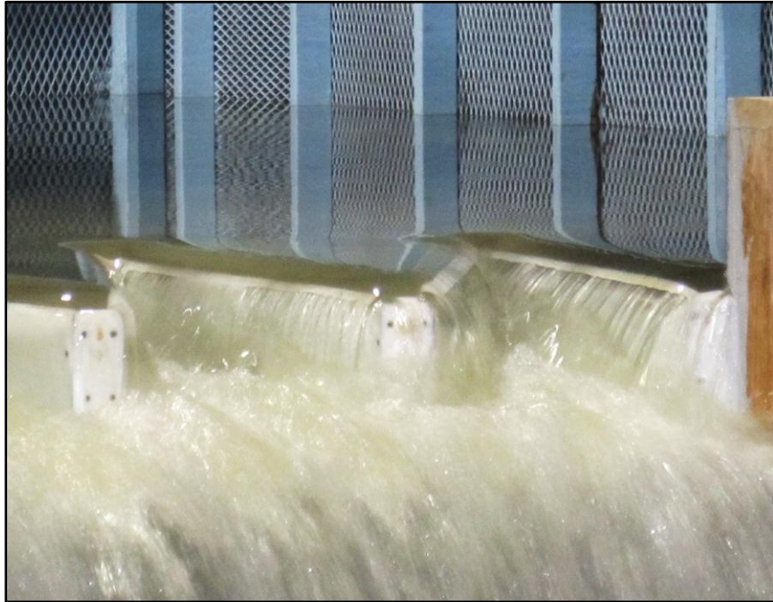
Fig. 23. Natural aeration of 1.5 cycles on \alpha = 12^\circ sidewalls ( H_T/P = 0.2 ).
