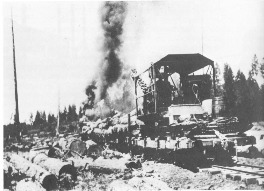
During McPhee's heyday, sixty miles of narrow-gauge logging railroad stretched into the timberland. Here a logging train, with mechanical loader at rear, departs the log loading point for McPhee. (C.W. Sward, U.S. Forest Service)
