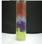
REMBRANT examines the affects of inertia on granular separation. The experiment includes two to four different bead sizes in one container that will be shaken and recorded to evaluate the ensuing collisions. Because of minimized gravitational effects, the granules will not be subject to buoyant or convective forces.
