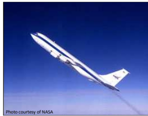
NASA's "vomit comet" simulates microgravity by flying a parabolic path.
