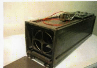
Picture of the PPOD deployment device, courtesy of www.cubesat.org .
