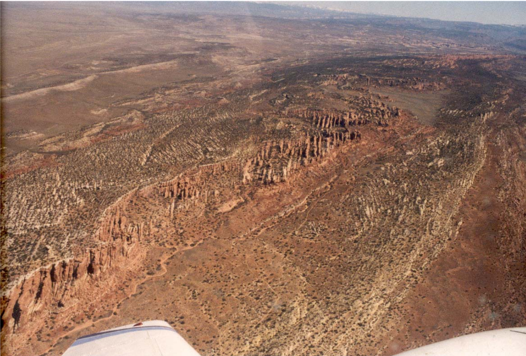
Figure 15: Fracture domain F. Aerial photograph of fractures within domain F. There is a distinct 30^{\circ} - 40^{\circ} variation in fracture strike between the Moab Member and the underlying Slickrock Member of the Entrada Sandstone. View is to the southeast.
