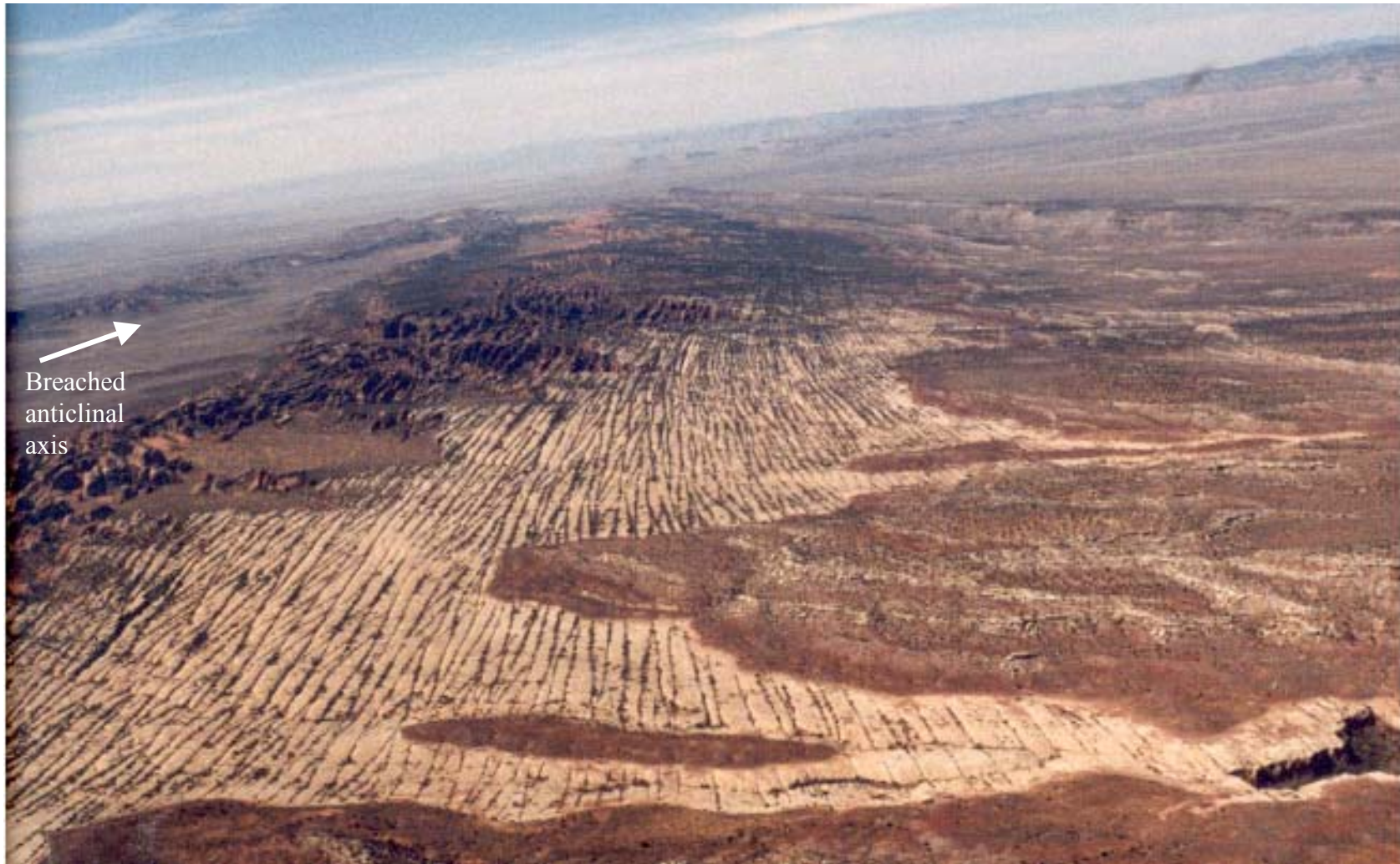
Figure 7A: Fracture domain B. Aerial photograph of fractures in domain B southeast of domain A. View is to the northwest, of a section of the northeastern anticlinal limb several km southeast of Figure 6A. Fractures here begin to fan out and strike up to 40^\circ oblique to bedding strike. Figure 7B illustrates how these fractures are due to fan-wise extension normal to the axis of a plunging anticline.
