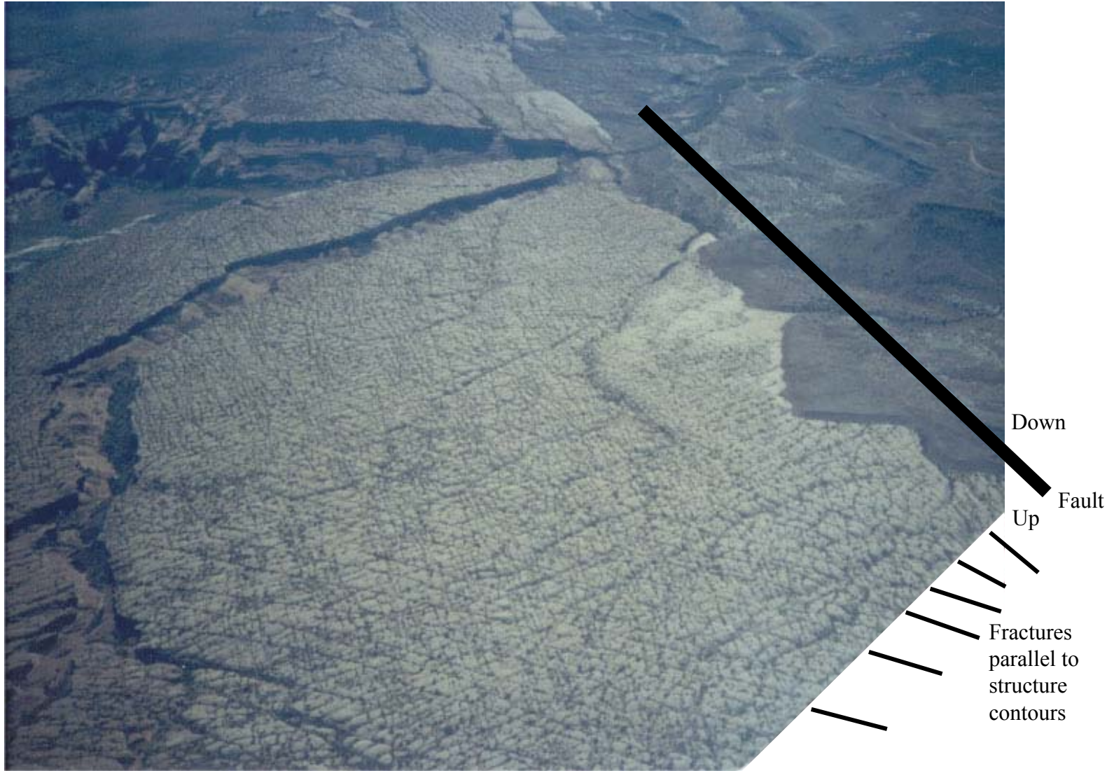
Figure 12: Fracture domain E. Aerial photograph of two fracture sets within domain E. One fracture set is parallel to structure contours the second is parallel to local faulting. View is to the east.
