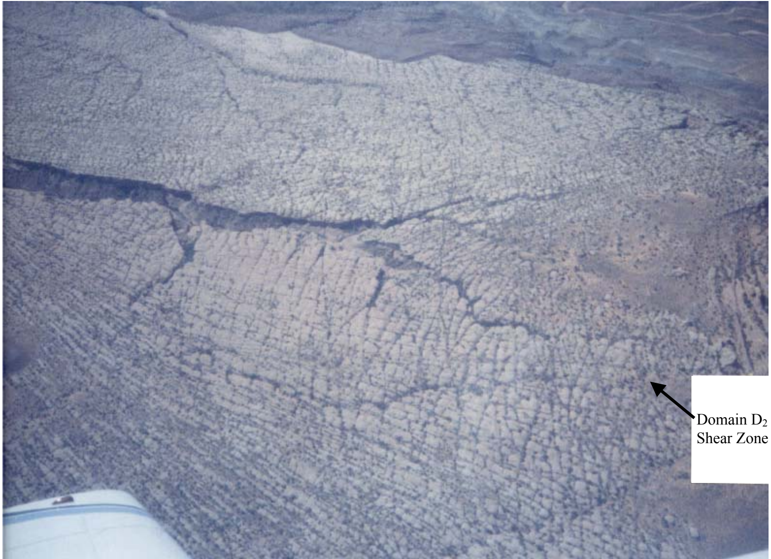
Figure 10B: Fracture domain D. Photograph showing the plan view orientation of possible conjugate shear fractures within domain D_2 . View is to the southeast.
