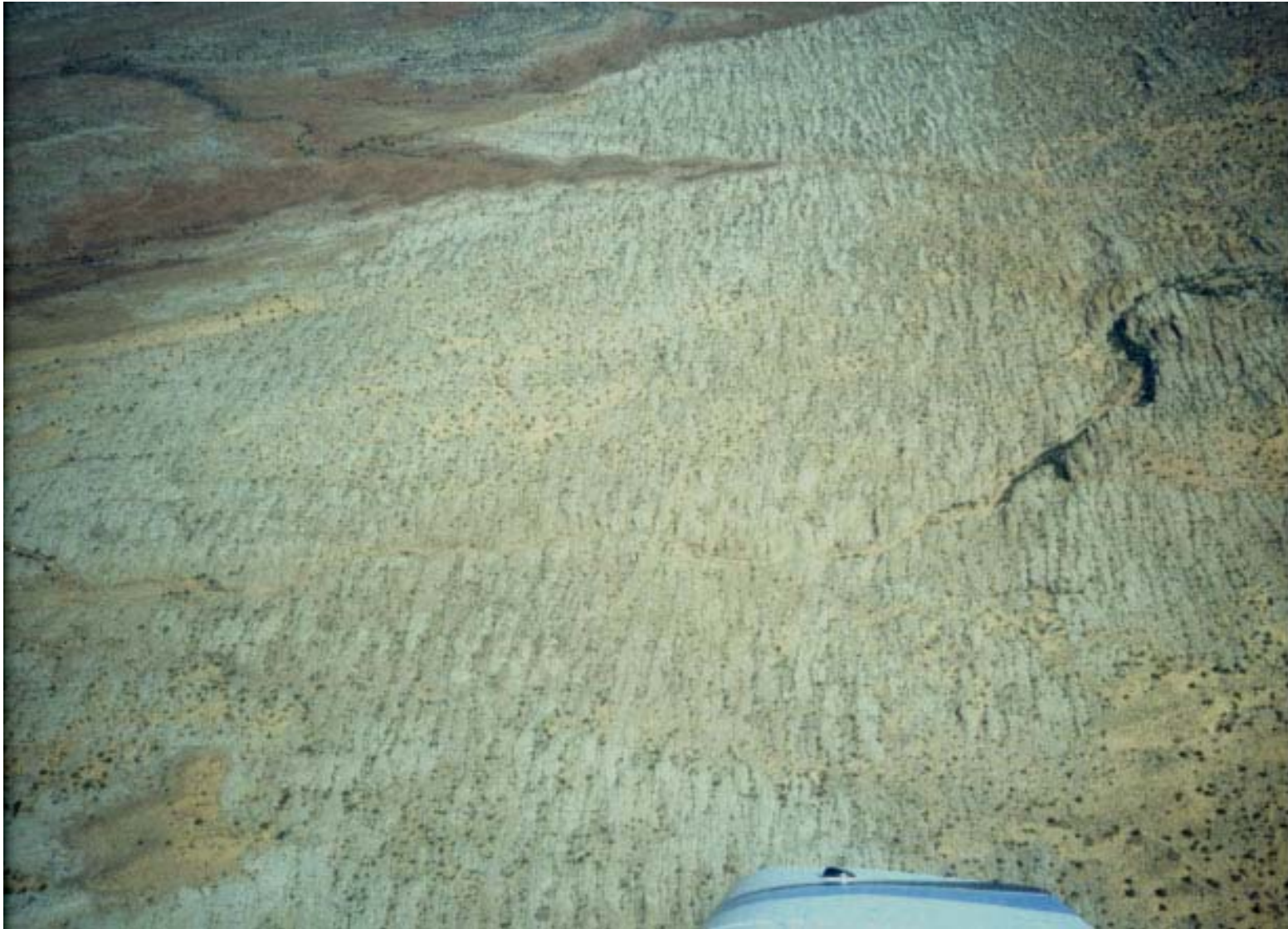
Figure 17: Aerial photograph of the Courthouse Syncline. Fractures within this broad syncline are parallel to the axis of the syncline. The fractures probably resulted from extension normal to the axis during subsidence driven by withdrawal of underlying evaporites.
