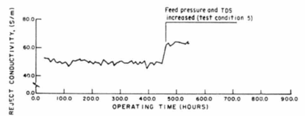
Figure 57 — The UOP membrane 1001 PA (PV-3) performance (sheet 1 of 2)
