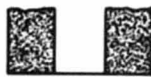
1. Have hole at least 0.3m(1ft) wider than ball diameter and 13cm(5in) deeper than ball.
