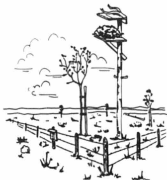
Figure 3.3-21. Diagram of artificial raptor nest platform with sunshade and perch mounted on utility pole (after Yoakum et al. 1980, modified from Olendorff and Stoddart 1974).
