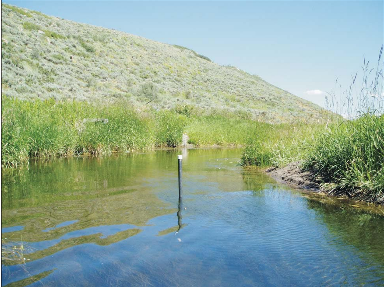
Figure 8. Streambed piezometer installed at site ECC-7, near Park City, Utah.
