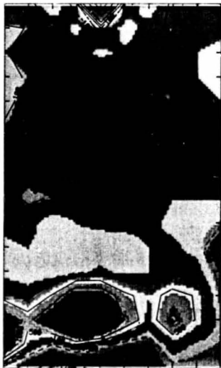
FIGURE 15. Level Sliced Color Map of Magnetic Data at Site 1.
