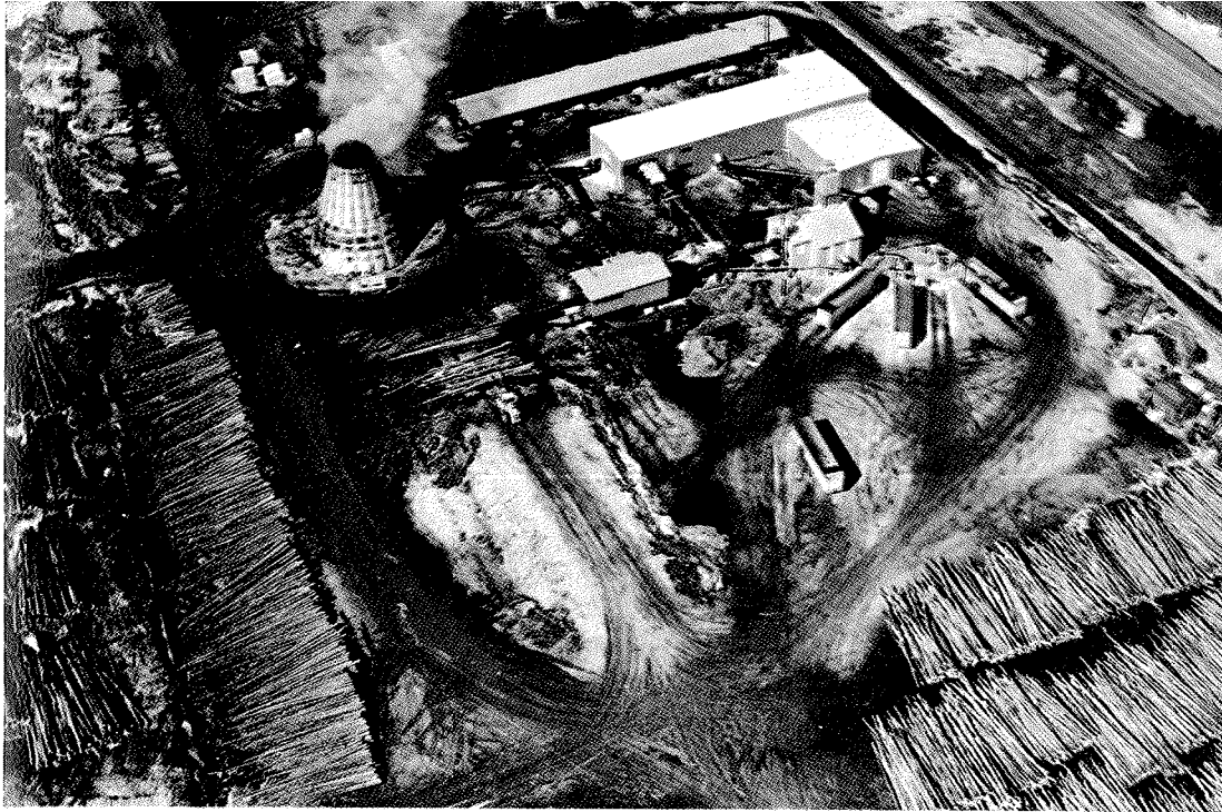
The Rajala Timber Company operates a large, modern saw-and-chip mill west of Deer River. The larger-diameter portions of tree length aspen logs are sawed into lumber. The smaller portions are debarked and chipped. Chips are now trucked to the Boise-Cascade mills at International Falls.
