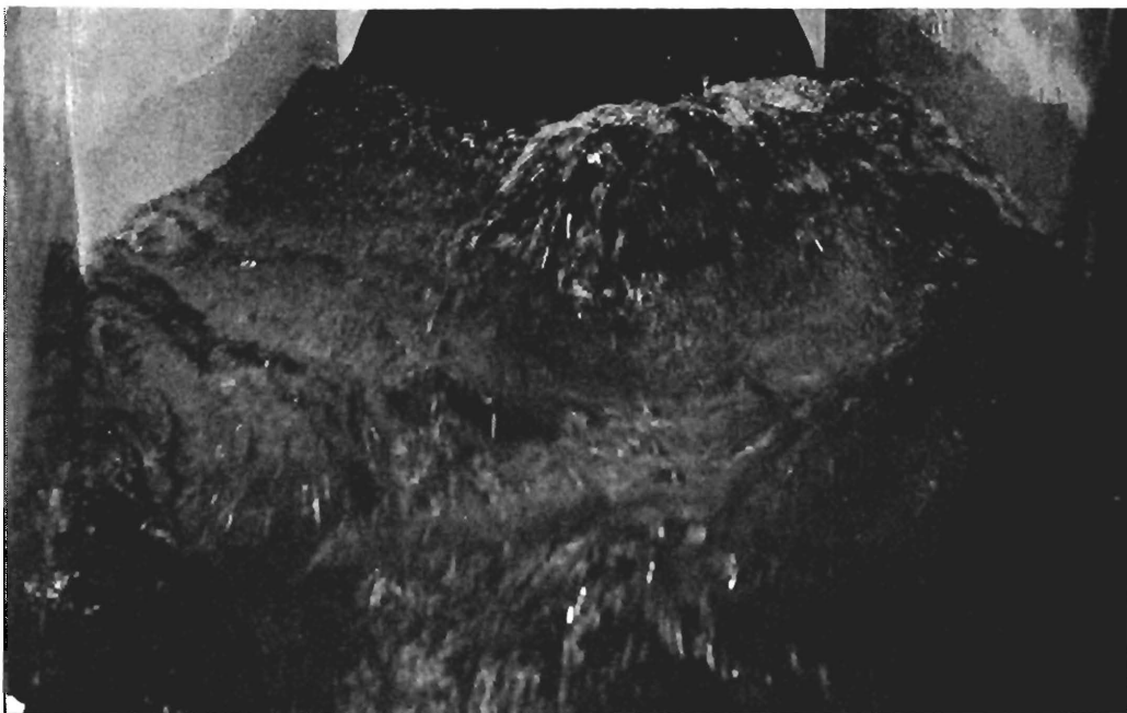
Figure 19. Typical view of high flow in the entrance section of the 18-inch Parshall flume. (Submerged flow, Q = 15 cfs, H_a = 2.02 ft, H_b = 1.82 ft, 90% submergence, the slope of the incoming concrete pipe = 0.0035, facing upstream.)
