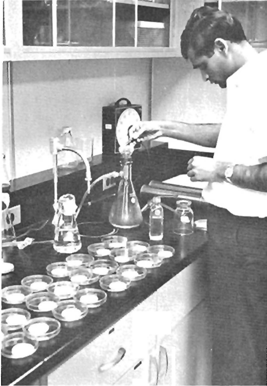
(d) Removing the filter paper aseptically from the filtering unit
