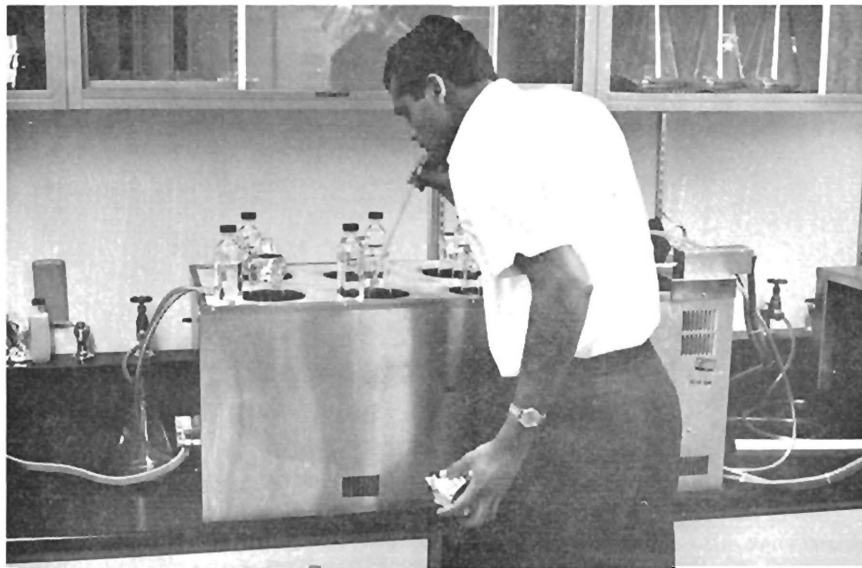
(a) Taking 1 ml sample from experimental flask
