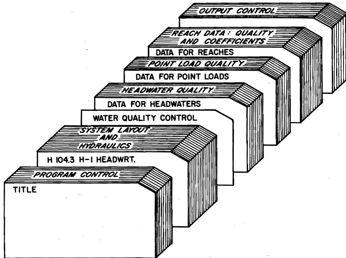
Figure A.1. Typical data deck setup for PSSAM.
