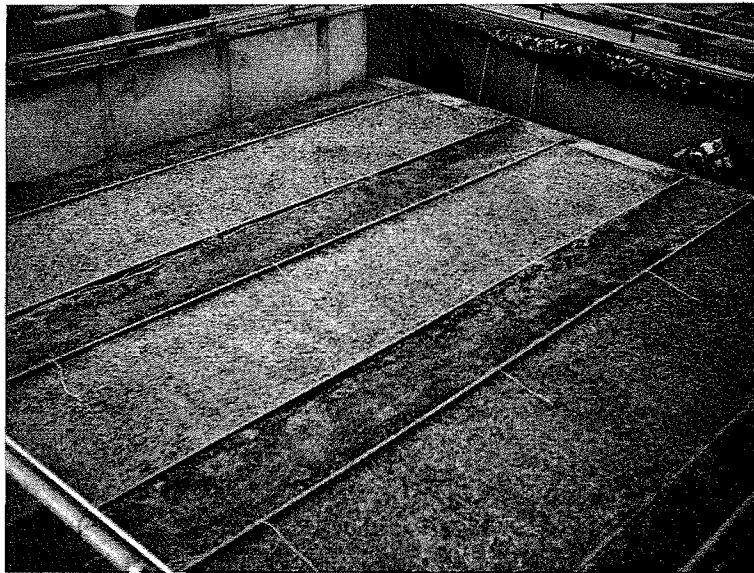
Figure 4. Mulched and seeded test plots after psychrometers are in place.
