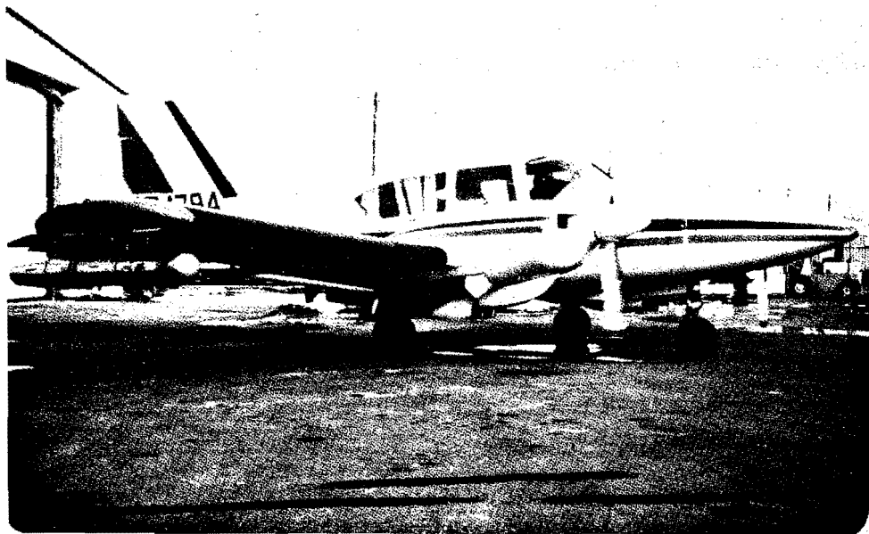
FIGURE 5.2. A Piper Aztec Aircraft Equipped for Aerial Cloud Seeding
