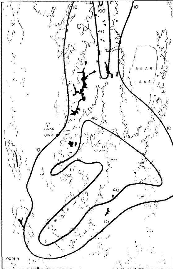
Figure 18a. Isopleths of silver concentration (gm/ml times 10-12) for snow samples taken following airborne seeding: FY 70.
