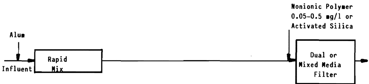
Figure 3. Flow sheet for typical direct filtration using alum and nonionic polymer or activated silica (Culp, 1977).
