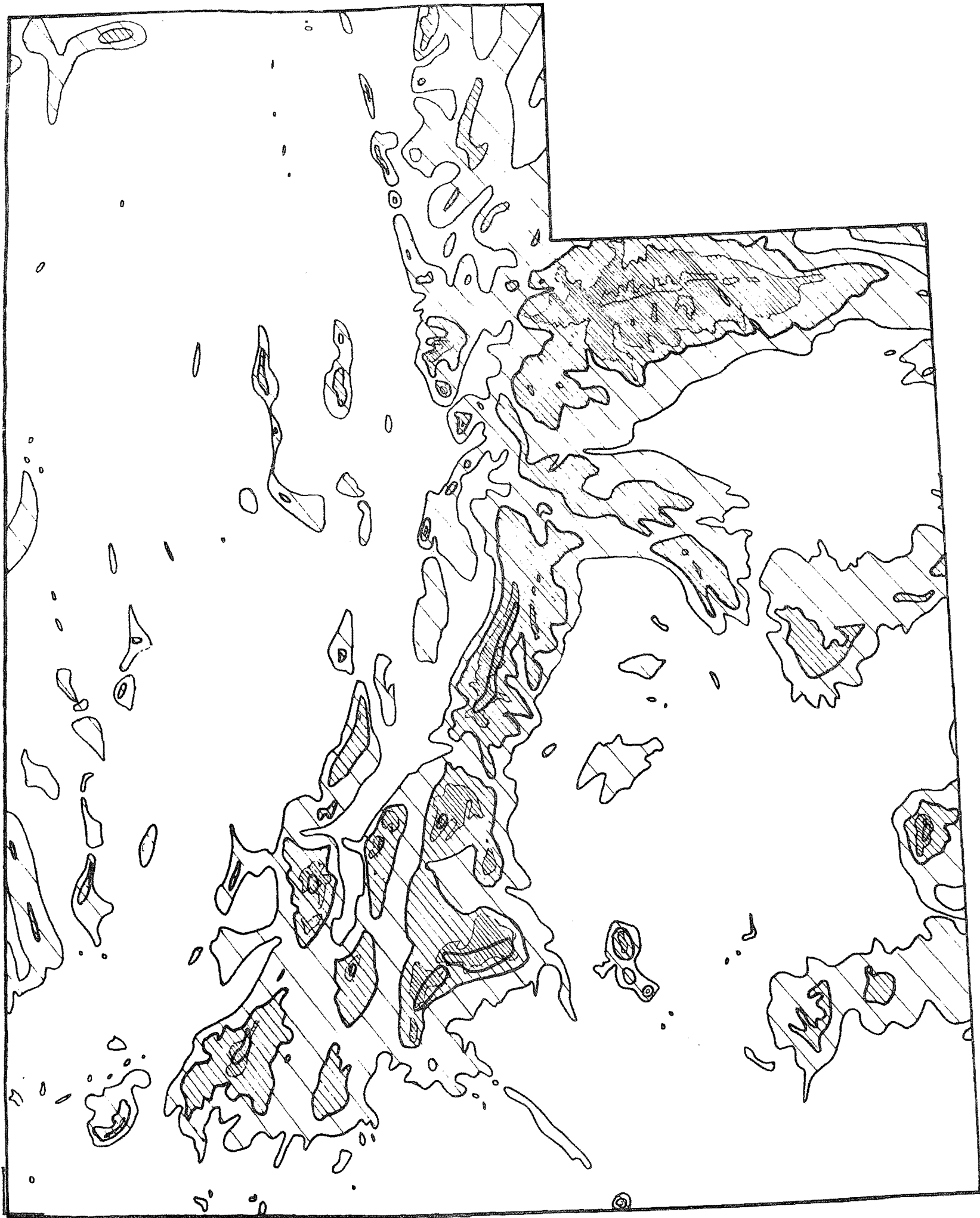
Figure 10. Median July precipitation enhancement resulting from seeding 32 percent of total precipitation with an assumed rate of increase of 50 percent of that precipitation. Contours, 0.3 inches.
