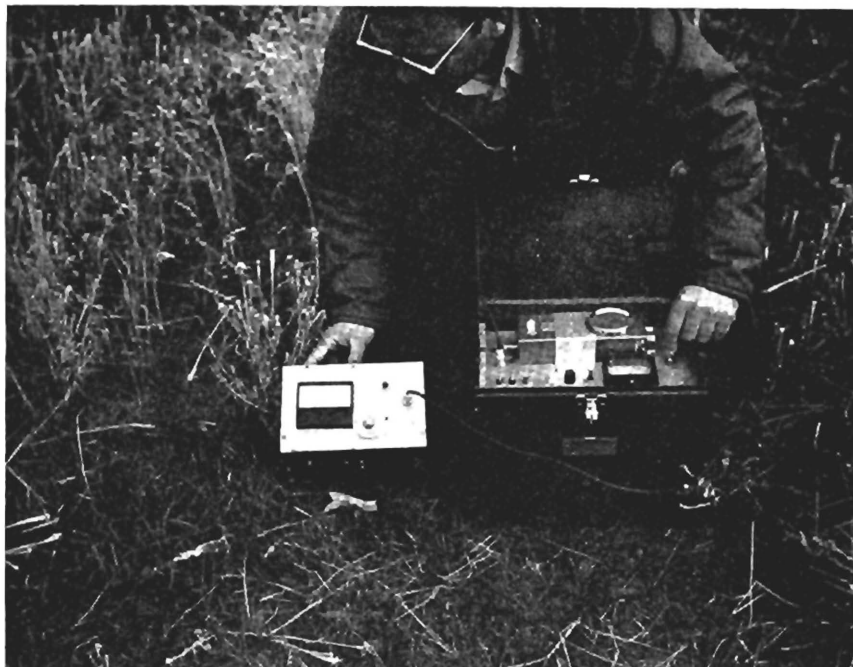
Figure 8. Photograph of 170 MHz transmitter, voltage regulator, and battery box.
