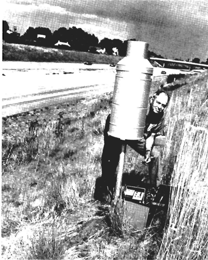
Figure 6. Typical weighing recording rain gage for measuring precipitation at the Layton site. The instruments at its base are the recorders for wind and soil moisture.
