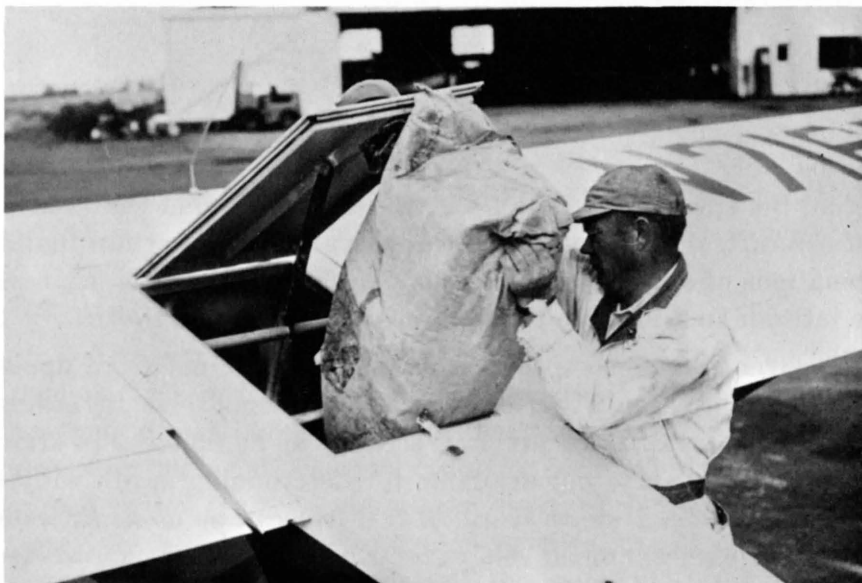
Figure 23. Loading hopper with powdered alcohol.
