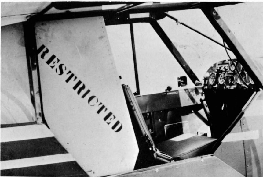
Figure 21. Hopper is located immediately behind pilot's seat.
