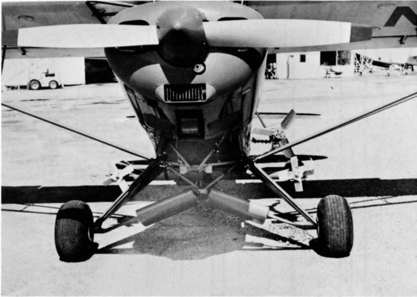
Figure 10. Forward view of new powder dispensing unit.
