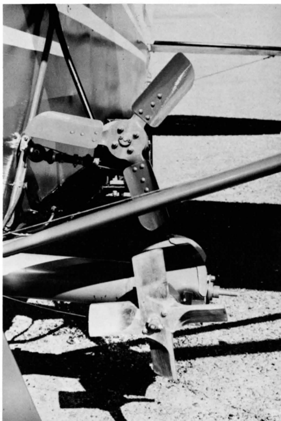
Figure 18. Brakes, operated by cables, have been installed on the agitator propeller (upper) and steel-wire brush propeller (lower).
