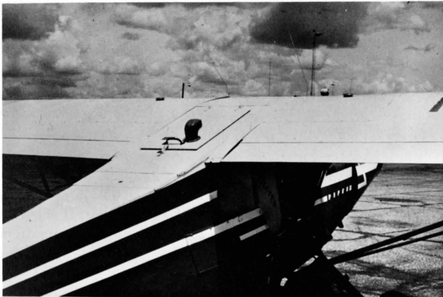
Figure 22. Air scoop is located on hopper lid.
