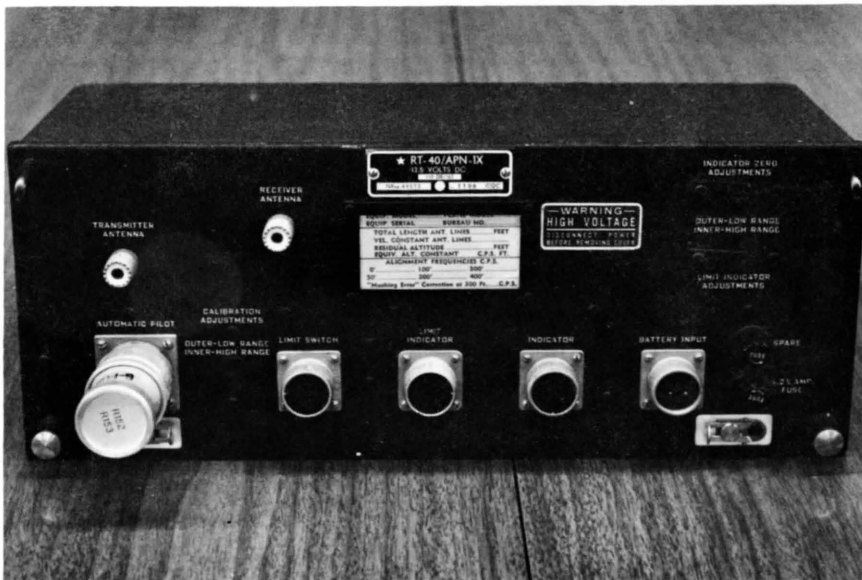
Figure 39. Transmitter-Receiver on AN/APN-1 radio altimeter.
