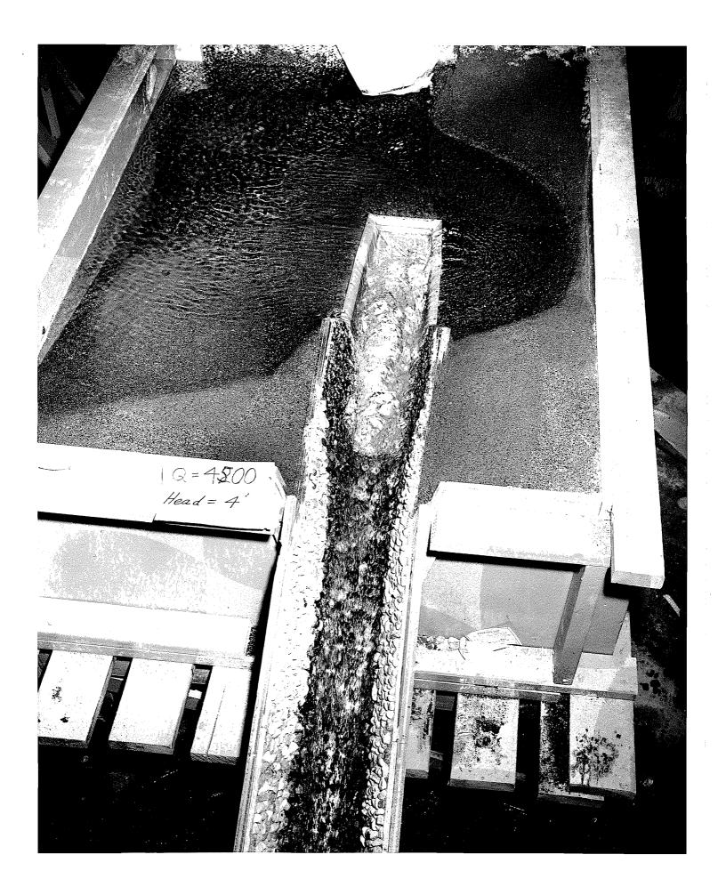
A view the same as Picture No. 3 but with no water running. The floor of the inlet is 24 feet wide and the side slopes are 1/4 to 1. The stones seen on the floor of the chute simulate two-foot average-height roughnesses on the prototype. The smaller roughnesses on the upstream side-walls would be approximately one foot high.
