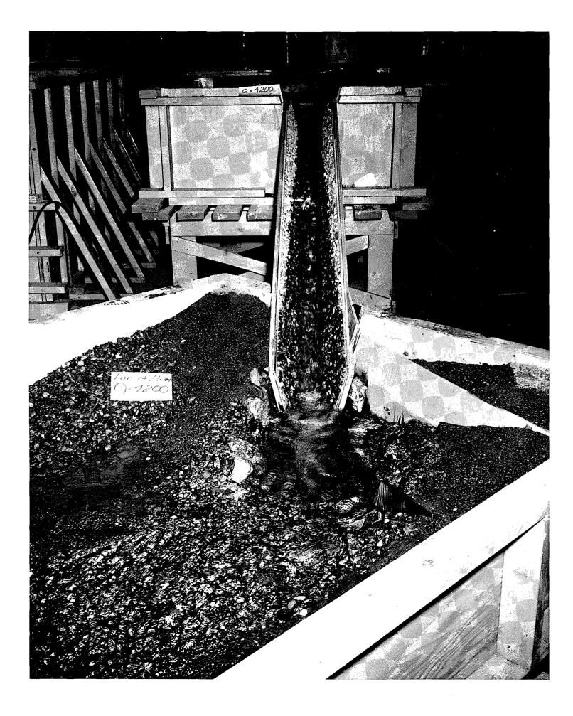
Water seen leaving the stilling basin still has considerable velocity. However, because bedrock is so close to the surface, no particular problem is expected with scour in this area.
