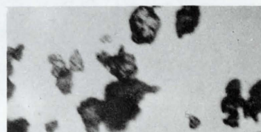
Powder D. Mean-diameter particle size 85 microns. This material was supplied commercially in flake form, cooled to from 25° to 35°F and then ground in a pulverizing machine as shown in Fig. 19. It emerged from the machine at a temperature of from 75° to 85°F. Some of this powder was transported in a station wagon in 50-pound bags for a distance of 800 miles and no objectionable lumping occurred.
