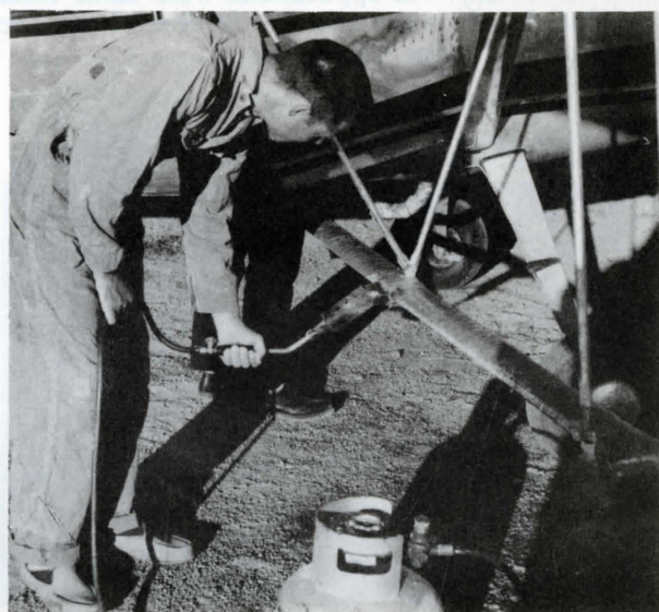
Fig. 15. Time required for pre-heating the booms and nozzles was decreased by supplementing the aircraft heat with heat from a propane torch.
