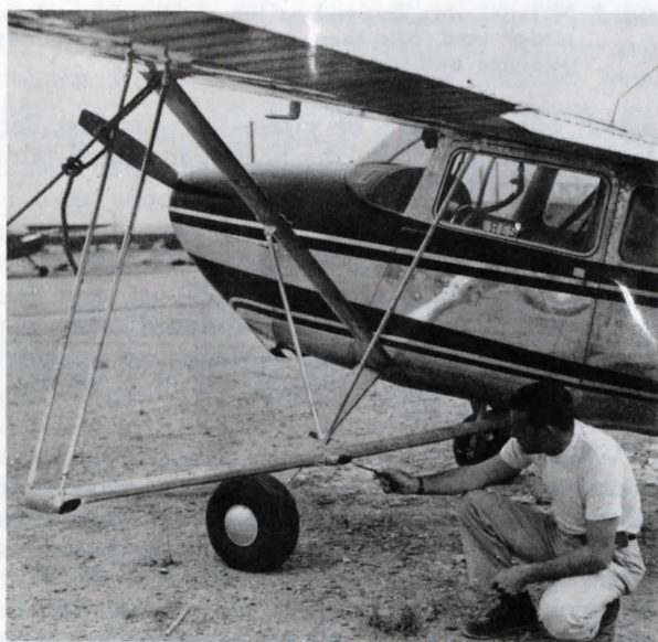
Fig. 4. Aluminum shrouding directs hot air around the booms and nozzles.
