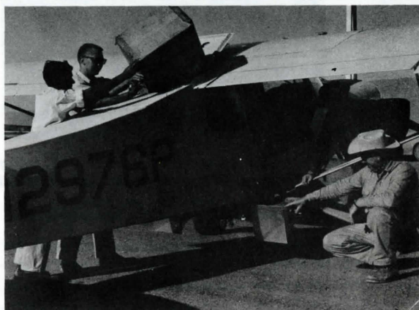
Fig. 9. A dusting plane equipped with the double-venturi dispenser is being loaded.
