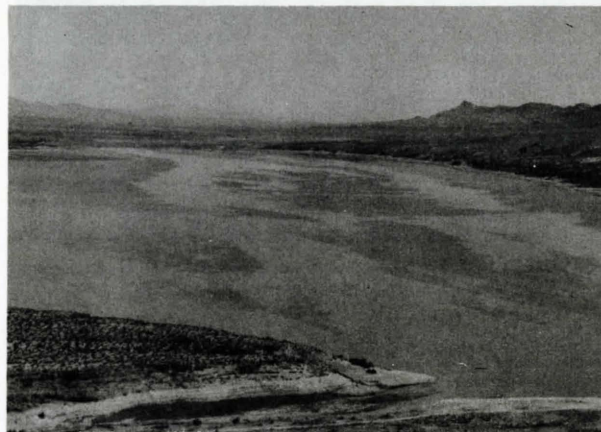
Fig. 28. Parallel strip-applications of powders and liquid were made to Caballo Reservoir for purposes of comparison.
