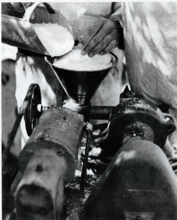
Fig. 19. Flaked hexadecanol was ground to a fine powder in a pulverizing machine.
