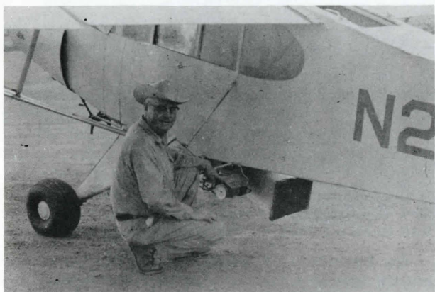
Fig. 7. The discharge end of the venturi tube was screened in an attempt to pulverize lumps in the chemical.
