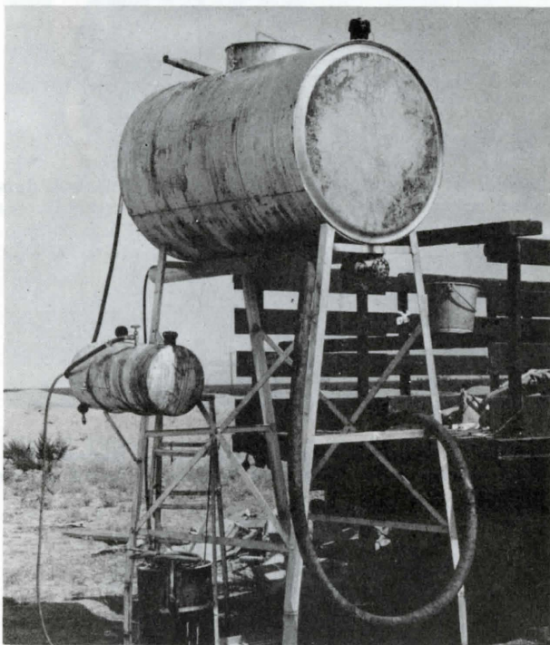
Fig. 13. Flaked evaporation-retarding chemical was melted in a large steel drum using kerosene-fueled burner for heat.
