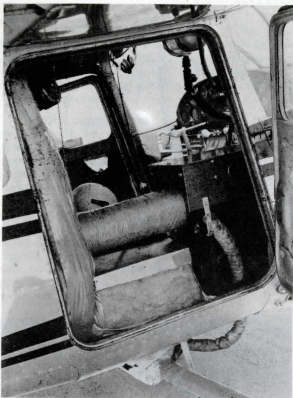
Fig. 3. A gasoline heater supplies hot air to the shrouded boom and nozzles to prevent their freezing.
