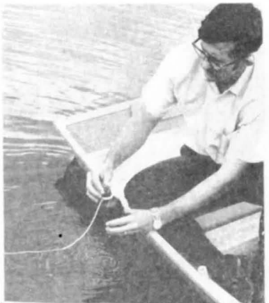
(g) Retrieving the reaction vessel after the equilibration period (15 mm) had lapsed.
