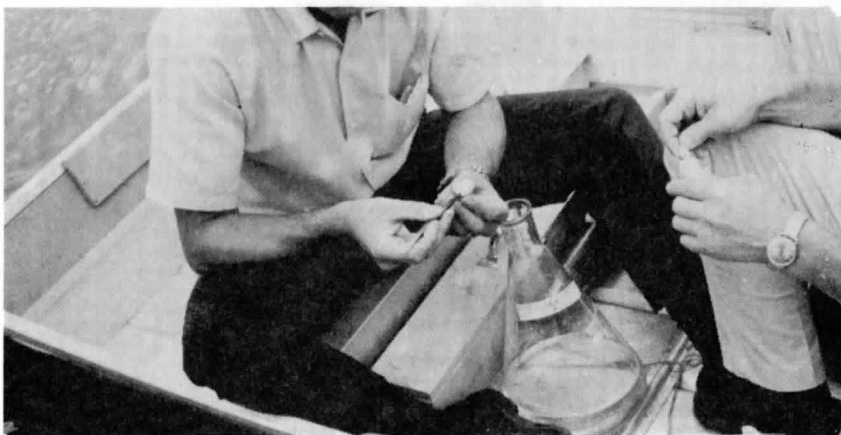
(p) Gluing the filter disc onto an aluminum planchet.
