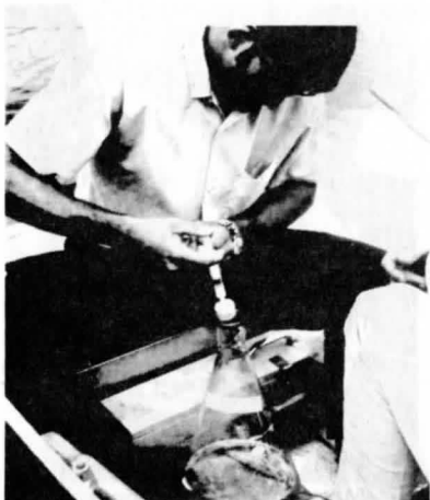
(m) Filtering the radioactive sample into a waste reservoir.
