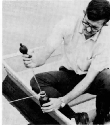
(h) Transfer the 5 ml radioactive glucose ( 1 \mu\text{ c/ml} ) or bicarbonate ( 0.5 \mu\text{ c/ml} ) solution to the reaction vessel.
