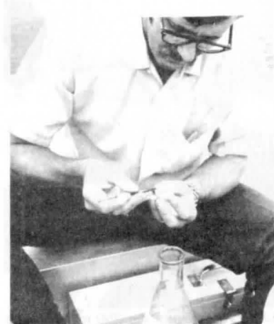
(o) Removing the radioactive filter disc from the Swinnex adapter with forceps.
