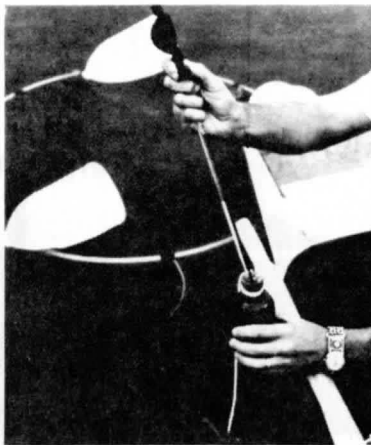
(k) Removing a 10 ml sample aliquot for radioactivity analysis.
