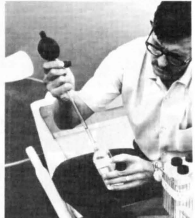
(f) Measuring 5 ml portions of the radioactive glucose or radioactive sodium bicarbonate solutions prior to transfer to the reaction vessels.
