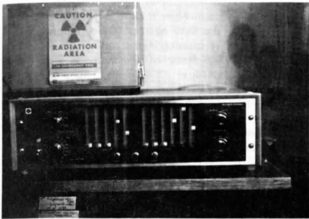
(a) Nuclear Chicago Beta Radiation Counter used for counting the radioactive emissions from the filter discs collected in the kinetic experiments.
