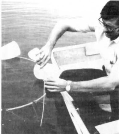
(d) Transferring the 250 ml measured volume to the reaction vessel.
