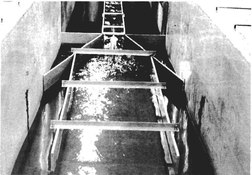
Fig. 18. View of downstream section with expansion ratio of 1:3 and B/b ratio of 3.
