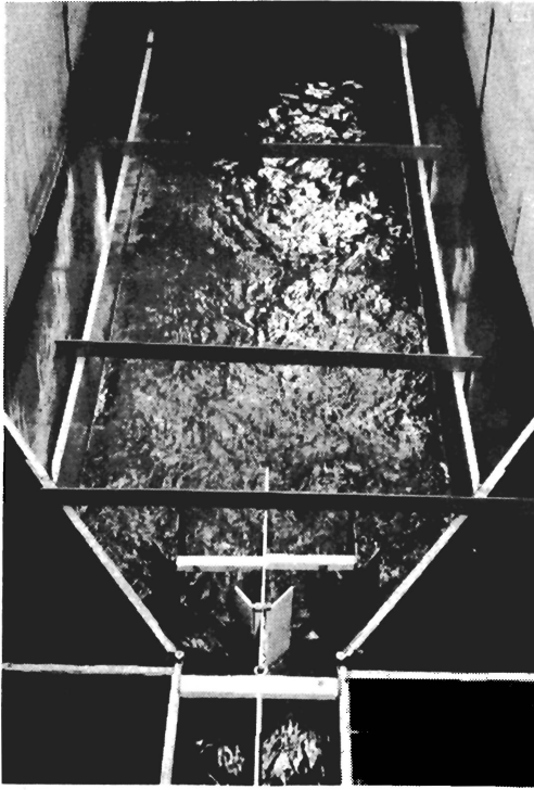
Fig. 29. Experimental flume with 2-3 expansion ratio and a B/b ratio of 3, operating with final baffle design.
