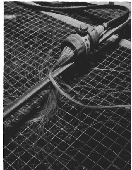
Items 11 and 12. Distribution head and tubing
