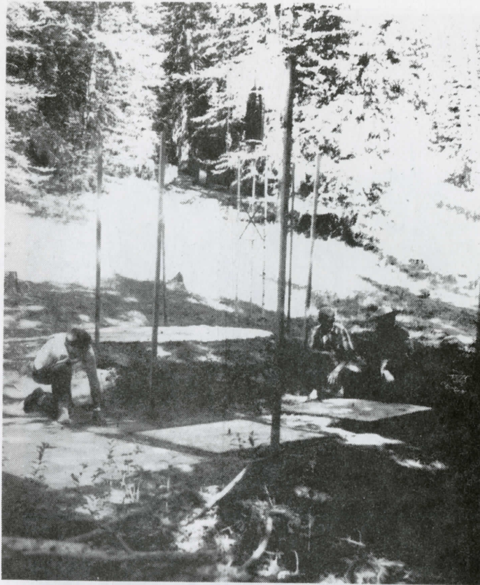
Figure 17. Providence Lake pillow test site. This site was abandoned after one year due to snow drifting problems.
