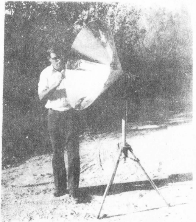
Figure 22. A sheet metal cone-type solar collector/concentrator. Three such units are required to power an 8 liter/minute pump.
