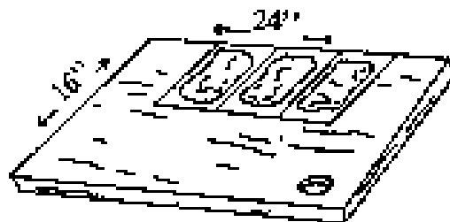
Figure 4. A glue trap to catch snakes indoors or under porches can be made by attaching rodent glue traps to a wooden board.
