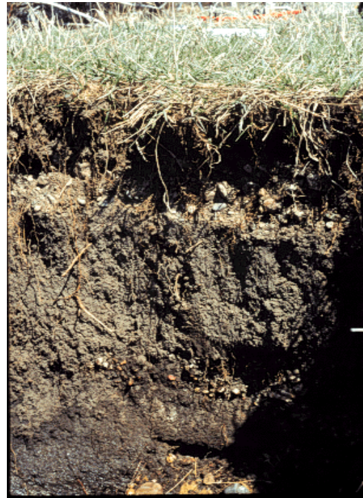
Photograph E Composite stream banks showing interspersed layers of coarse gravel with fine-grained sediment. Note the presence of more than one coarse layer in the stream bank.
