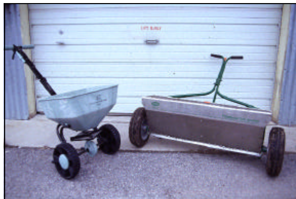
Figure 3. Rotary (left) and drop (right) fertilizer spreaders.
