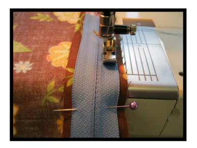
STEP 3: Replace sewing machine foot with a zipper foot. Place zipper face down with the teeth centered on the pressed open seam on the inside of the garment, matching top and bottom stops with marks.
