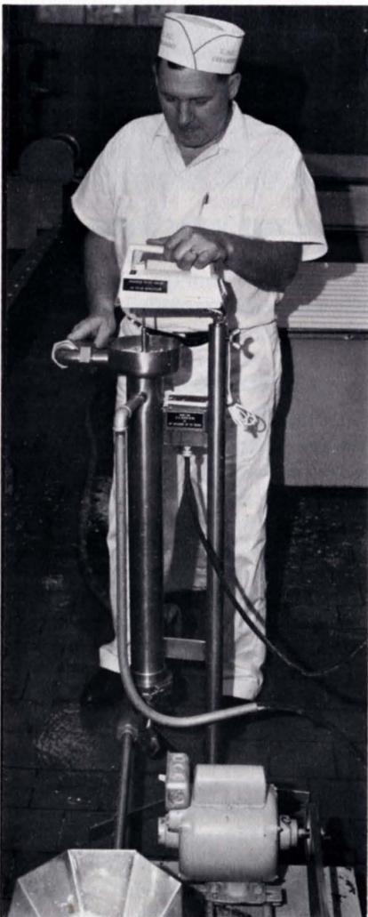
Figure 1. Cottage cheese, usually made in large batches, can now be manufactured in a continuous process by using equipment and methods designed by Dr. Anthon Ernstrom of USU. One commercial unit now in operation on an experimental basis produces 3,000 lbs. of finished cottage cheese per hour.
