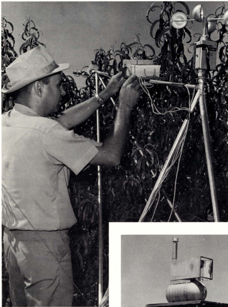
Figure 3. Instruments are set up at tree-top level to measure air currents and temperatures. By better understanding these factors more effective orchard heating methods can be devised.
