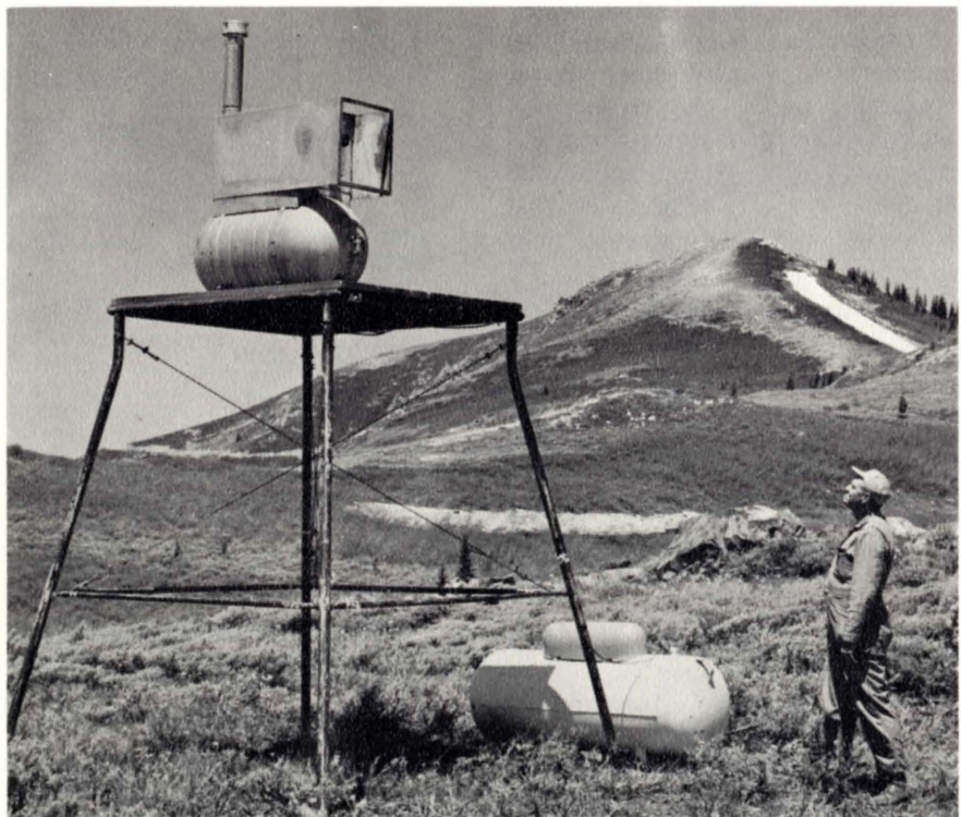
Figure 4. This remote-controlled silver-iodide generator is used in the weather control studies at USU. Located high in the Wasatch Mountains this generator can be turned on by radio signal when cloud and wind conditions are conducive to cloud seeding.
