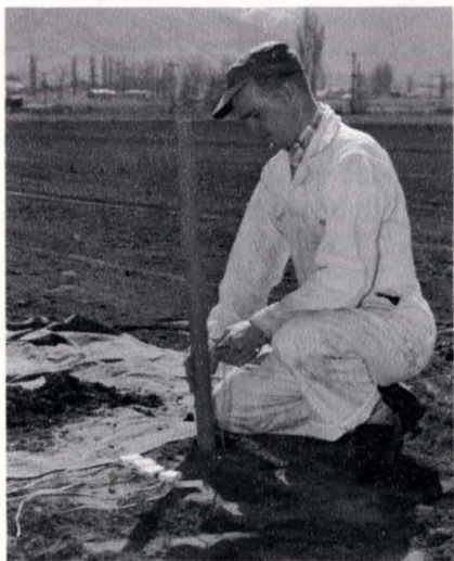
Figure 8. Resistance blocks being installed. They remain buried and the water potential can be "read" when the meter is attached.
