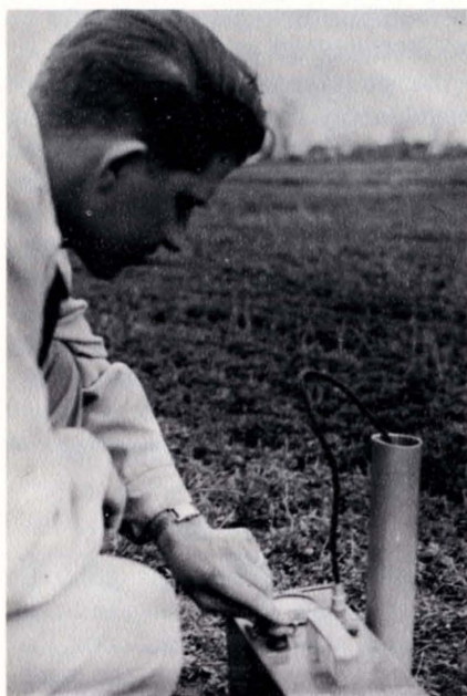
Figure 3. Using a neutron meter to measure the amount of water in the soil. The probe has been inserted into the tube.
