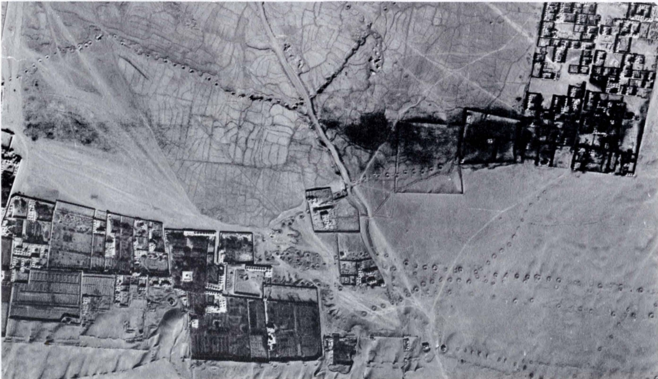
Figure 2. This air view clearly shows the ventilation and repair shafts which are sunk along the line of underground ghanats. As shown, many ghanats run right under the villages.
