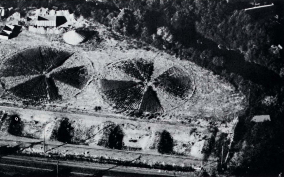
FIGURE 1. Site location layout of the 2-day (left) and 4-day (right) Point Source circles at the USU Agricultural and Irrigation Engineering River Lab. (Summer 1982).
