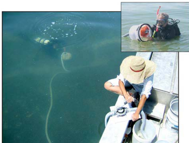
Figure 2 —SCUBA diver sampling biostromes in Great Salt Lake with a pump sampler. The inset shows the detail of the bucket and scrub brush used to dislodge brine flies so that they can be pumped to the surface.
