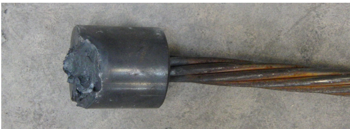
Fig. 13 Cable and chuck after being removed from specimen
