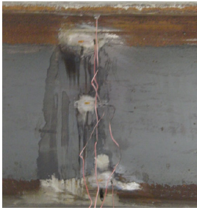
Fig. 6 Picture of strain gages installed on girder
