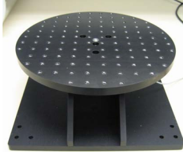
Figure 17: Oscillating Table for MOI measurements
