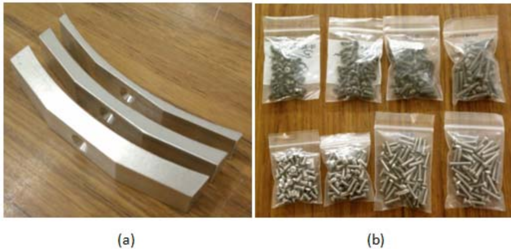
Figure 9: Balancing Weights a) Large weights for “rough” balancing, b) Small weights for “fine tuning”
