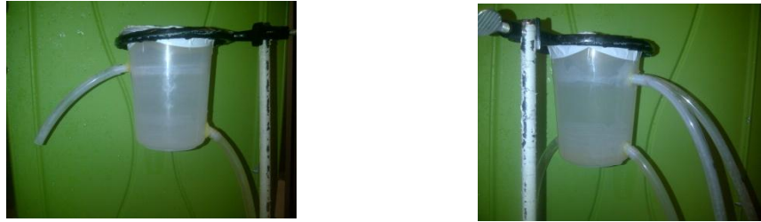
Figure 12 - Photograph of the downstream (left) and upstream (right) flow regulators
