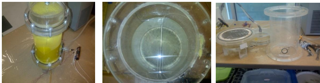
Figure 10 - Photograph of the side view (left), uncovered aerial view (center) and the individual components (right) of the flow cell.
