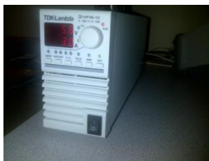
Figure 16 - Photograph of the constant-current power supply unit
