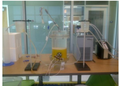
Figure 4 - Schematic and photograph the no-flow (static) experimental setup with the flow regulators elevated to the same height.
