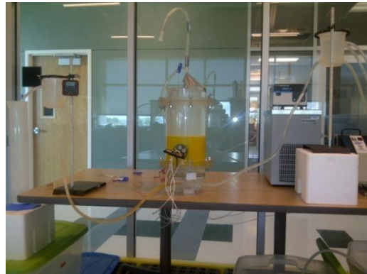
Figure 5 - Schematic and photograph the flow experimental setup with an elevation difference between upstream and downstream flow regulators.
