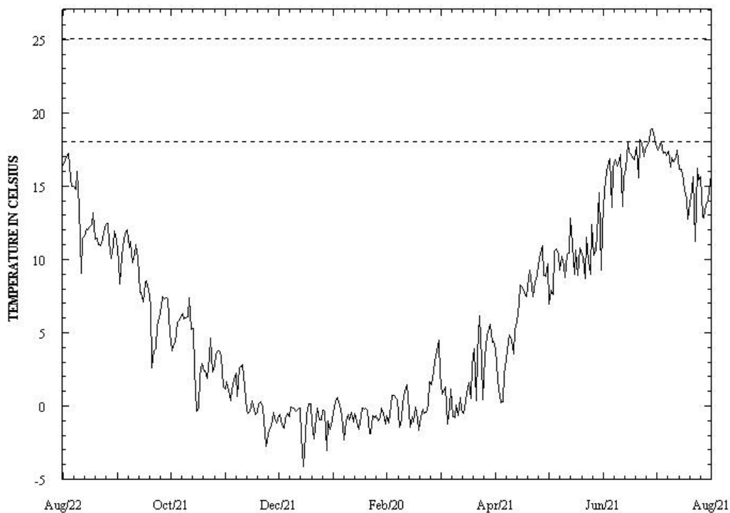
Figure 21: Temperature in Celsius recorded at U.S. Route 40 Bridge for 2009 and 2010 water years. The dashed line represents a zone of temperature where Bonneville cutthroat trout begin to show signs of stress and higher mortality rates (e.g., 18°C to 25°C) as a result of high summertime temperatures (Johnstone and Rahel, 2003).
