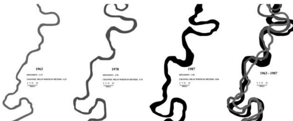
Figure 5. Polygons of the active channel from a section of the upper Strawberry River, from aerial photographs of 1963, 1978, and 1987, illustrating the increase in channel sinuosity and width in the 1970s and 1980s.
