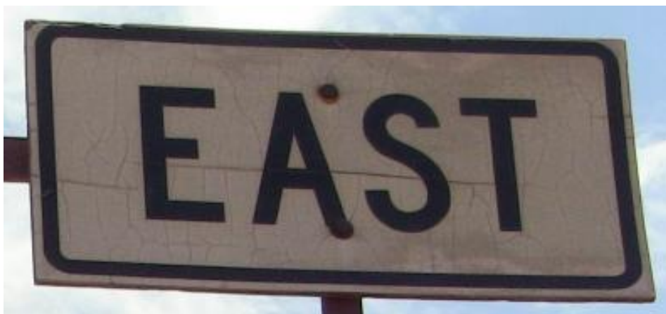
Figure 4.2 Type I cracking example.
