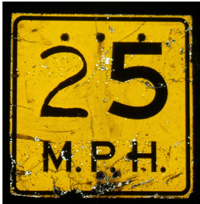
Figure 4.11 Bullet hole damage.
