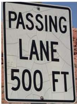
D. Cracking Damage
