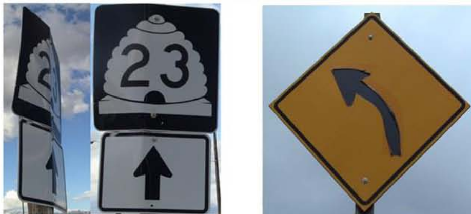
A. Bending Damage
