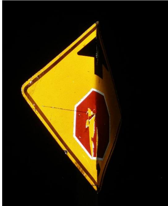
Figure 4.13 Issues presented with bending damage on prismatic sheeting.
