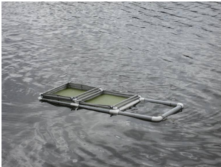
Figure 22. PVC frame with three 0.33 m 2 cells for duckweed field growth study.
