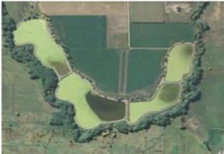
Figure 3. Duckweed on 23 ha (56-acres) of Wellsville Municipal Sewage Lagoons, which sit in a hollow. Furthest right lagoon is effluent side. ( www.maps.google.com )
