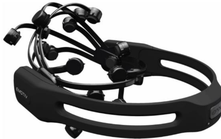
Figure 3-1. Original Emotiv EPOC ® neuroheadset with 14 electrodes and acquisition unit. 116
