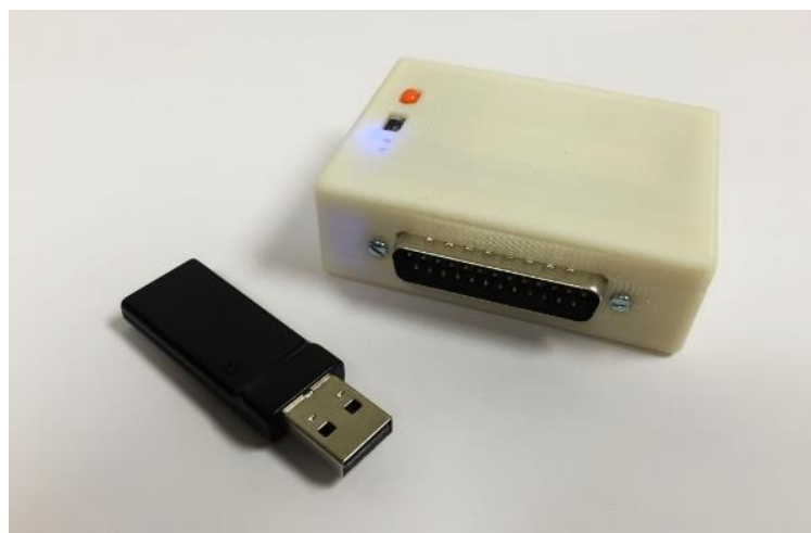
Figure 3-4. Plastic enclosure containing the wireless acquisition unit. A 25-pin D-sub connector allows the connection to the gold cup electrodes. The black USB dongle serves as the receiver of the streamed data.
