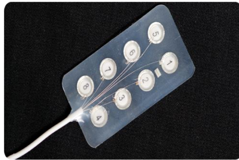
Figure 2.7: Subdural strip with eight electrodes [40]
